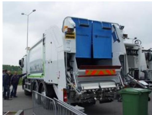
Lorry with rear loading facility Source picture: Geesink Norba
